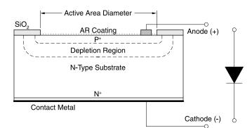
Figure 1. Planar diffused silicon photodiode
