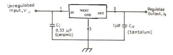
Figure 5.10 Negative fixed voltage regulator
