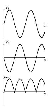
Figure 5.6 Full-wave rectifier waveforms
