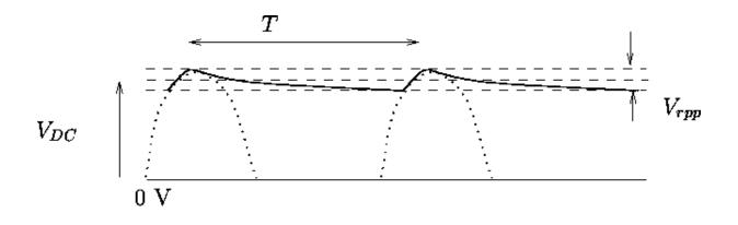
Figure 5.8 Filtered Half-wave rectified waveform showing  $V_{rpp}$  and  $V_{DC}$ .
