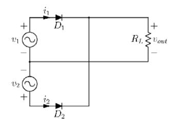
Figure 5.5 Center-tapped full-wave rectifier.
