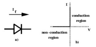
Figure a)Schematic symbol for a diode and b) current versus voltage for an ideal diode
