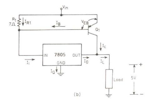
Figure 5.13 Fixed voltage regulator
