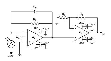
Figure 8. Photoconductive mode of operation circuit example: Low Light Level / Wide Bandwidth
