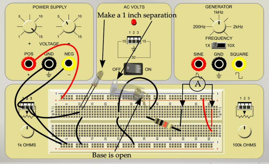
11. Turn on the power and repeat all the measurements for the various lamp voltages in the data table and set your meter to the 2.5 mA range
