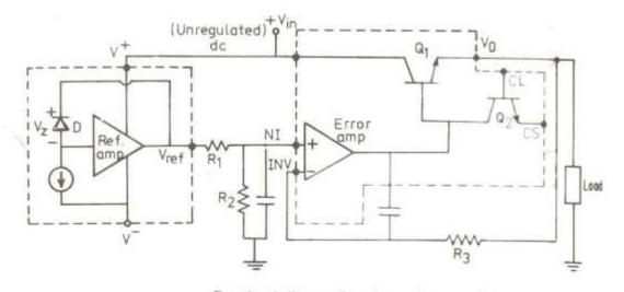
Functional diagram for a low voltage regulator  $V_{ref} \approx 7V$ ,  $V_0 = V_{NI} = 7R_2/(R_1 + R_2)$ ,  $V^+ = +V_{ee}$ ,  $R_3 = R_1 \parallel R_2$  (minimum drift),  $V^- =$ Gnd.
