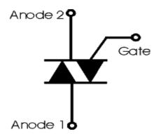
On the triac, the gate that acts as the trigger to turn the device on. The current then flows betweent he two anodes or main terminals. These are usually designated Anode 1 and Anode 2 or Main Terminal 1 and Main Terminal 2 (MT1 and MT2).
