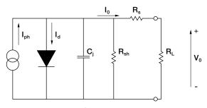
Figure 3. Equivalent Circuit for the silicon photodiode
