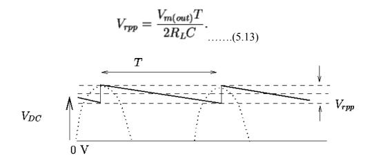
Figure 5.9 Approximate (triangular) filtered Half-wave rectified waveform
