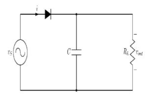
Figure 5.7 Filtered Half-wave rectifier.
