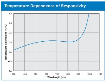
Figure 6. Typical Temperature Coefficient of Responsivity For Silicon Photodiode
