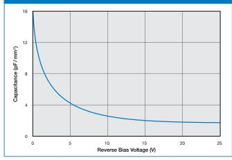
Figure 4. Capacitance of Photoconductive Devices versus Reverse Bias Voltage
