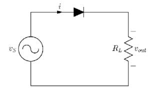
**Figure 5.3 Half-wave rectifier**
