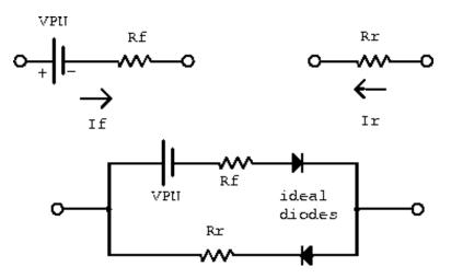
Figure 5.2 Equivalent circuit model of a junction diode
