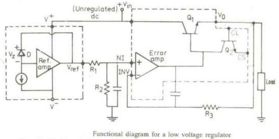
$V_{\text{ref}} \approx 7V$ ,  $V_0 = V_{\text{NI}} = 7R_2/(R_1 + R_2)$ ,  $V^+ = +V_{\text{cc}}$ ,  $R_3 = R_1 \parallel R_2$  (minimum drift),  $V^- = \text{Gad}$ .
